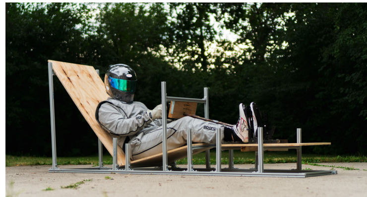
A brand-new driver jig, built from T-slotted aluminum, allows for infinite adjustability and reusability for many years to come!
