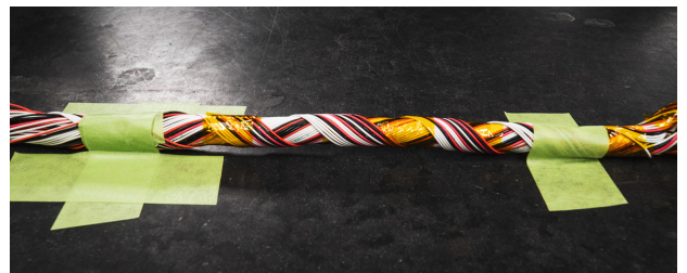
The wiring harness has been designed, cut, and twisted. Thanks to BMRS Wired for sponsoring material, and Rapid Harness for design software!
