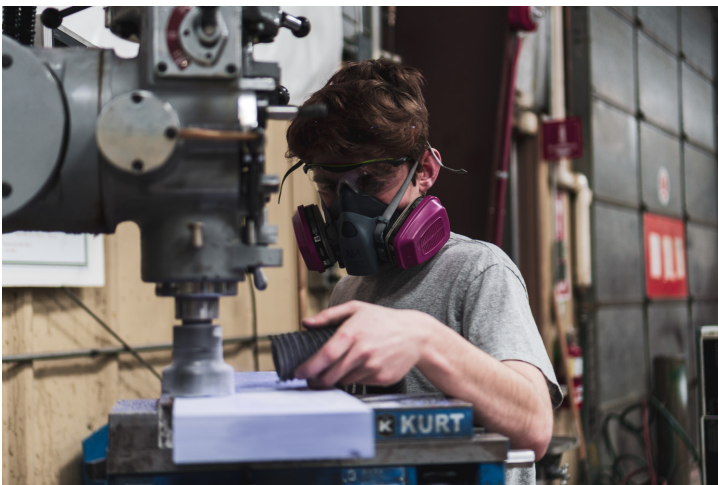
Ergonomics Lead, Andrew McNamara, helps machine a tooling board blank for aerodynamics mold CNCing.
