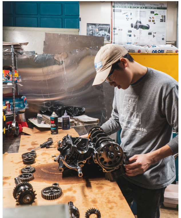
Powertrain Lead, Justin Yan, works on modifying the stock engine transmission during the engine rebuild.
