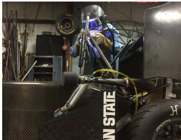
Brandon welding rear wing tabs for Car 16
