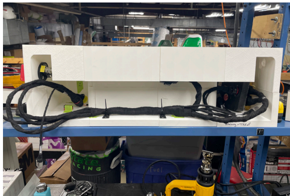
A 3D-printed part of the chassis used for wiring
