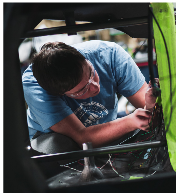
Nicholas Kopec installing Car 38's wire harness
