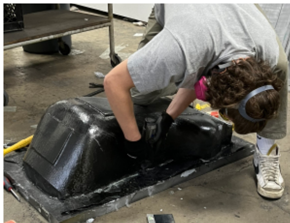
Calum Walton, the Rear Box and Manufacturing lead, assisting in popping the seat out of the mold
