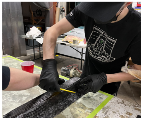
Suspension Lead, Nicholas Coubard, laying up the steering rack cover
