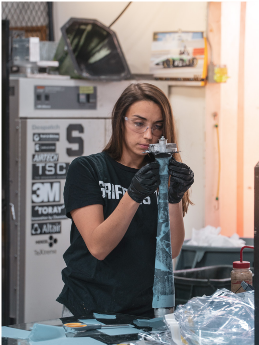
Intake & Exhaust Lead, Olivia Reyes, lays down a layer of release film during the intake diffuser layup
