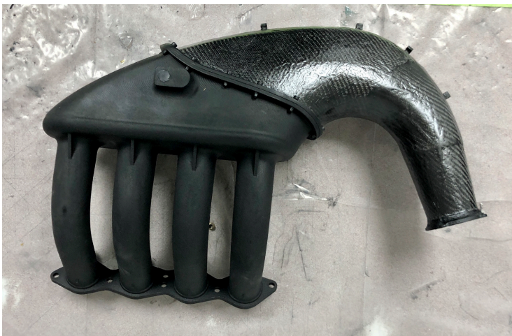
Ford did an amazing job 3D printing our intake this year. We can't thank them enough for their support!
