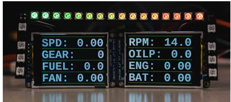
Our custom driver display is always an eye-catcher! This year the hardware and software were both completely redesigned (PCBs manufactured by Saturn Electronics Corporation!)
