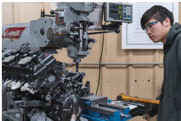
Justin Yan mills down our engine to fit the rear damper termination mounts
